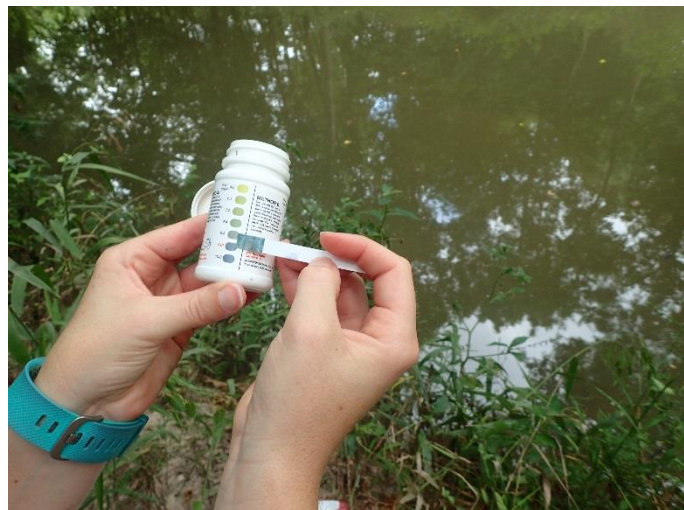
Figure 55. Chlorine test strip result for Upper Panther Branch sample 004
