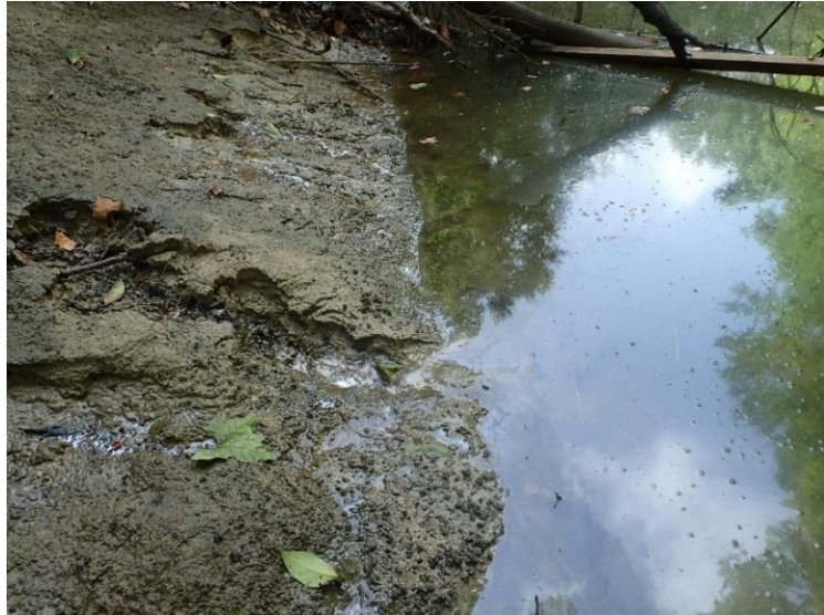
Figure 31. Groundwater discharge and surface sheen at sample 033
