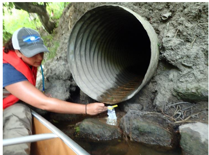
Figure 7. Collecting sample from discharging outfall
