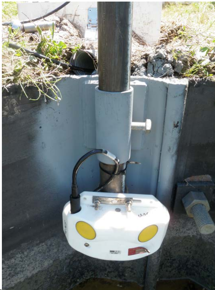
Figure 2. Sontek Argonaut SL1500 and associated bracket at USGS streamflow gaging station 08067252 Trinity River at Wallisville, TX.
