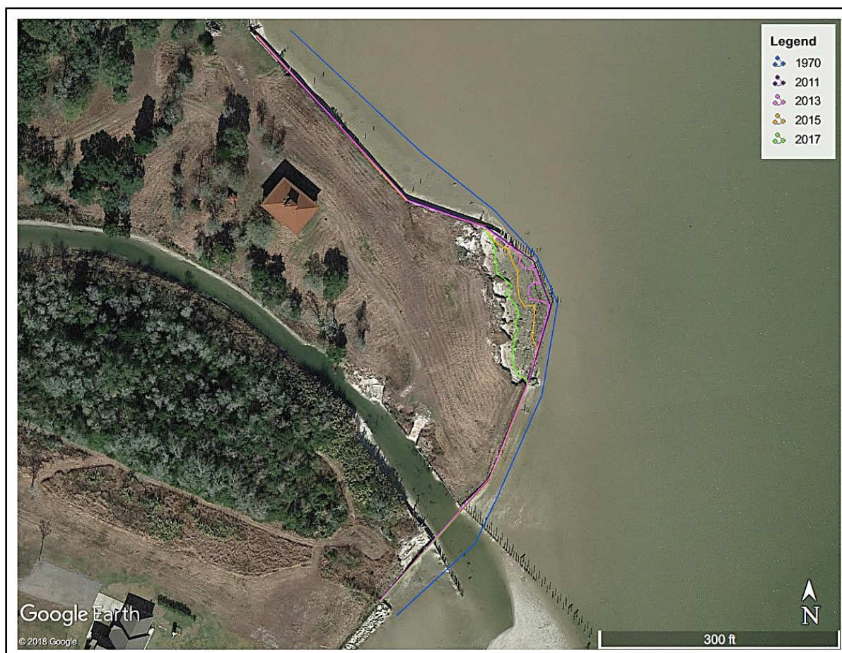
Figure 1. Approximate locations of Trinity Bay Discovery Center shoreline over time, indicating erosion on southeastern point since the failure of the bulkhead in 2012.
