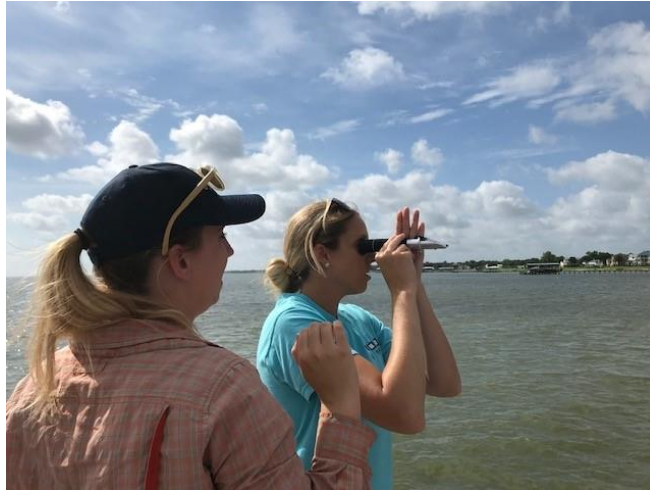
Checking water salinity with a refractometer
