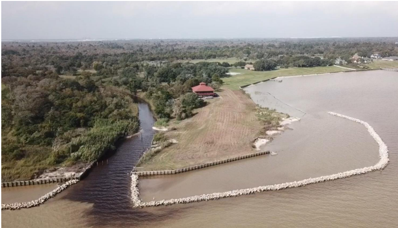
Figure 2. Aerial view of complete TBDC rip-rap breakwater and 300-foot oyster shell breakwater (photo credit: Galveston Bay Foundation).
