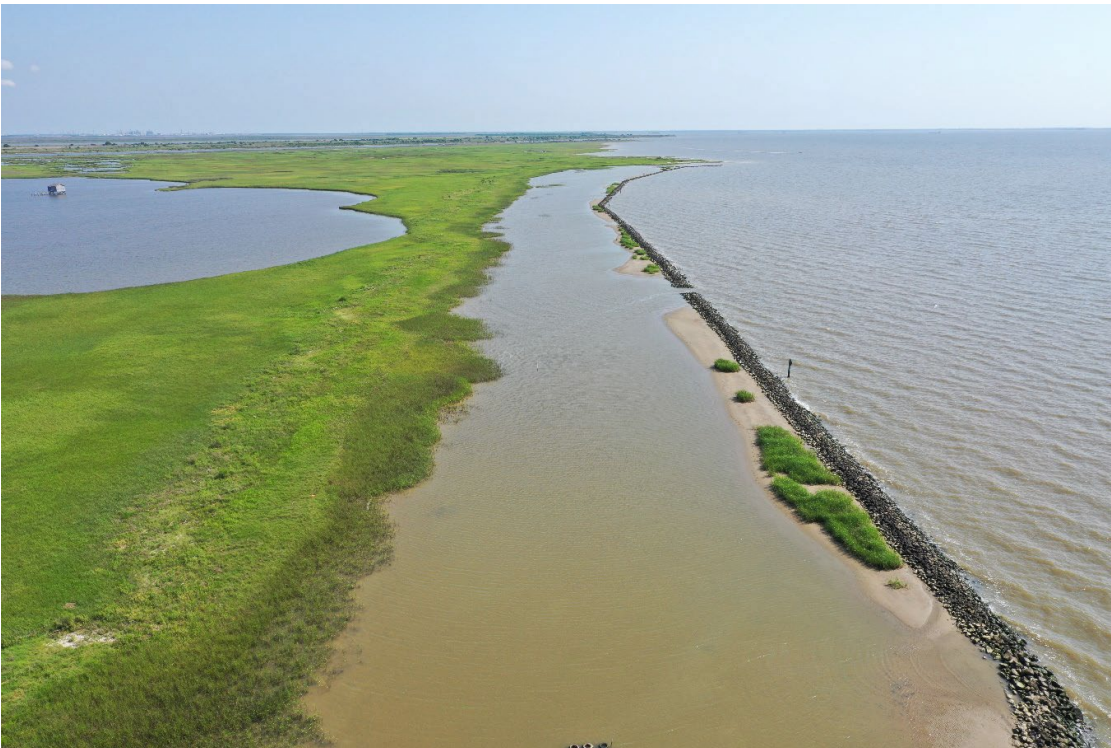
June 2021 photo looking to north. This is a reference to the first photo in this collection of photos. Notice the accretion of sediment behind breakwaters and the established intertidal fringe marsh (smooth cordgrass) and the natural expansion of the intermediate marsh. Photo of Phase II.
