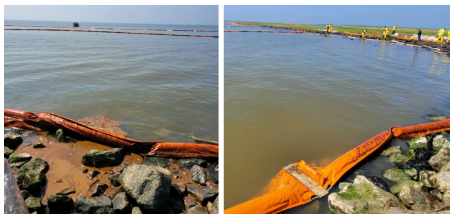
Fig. 2. Photos taken of the slicked VGO site. The site sampled was the most heavily slicked and is also indicated by the red arrows in Fig. 1. Up to 2 Liters of slicked oil was sampled along the shoreline and is stored at -20°C for subsequent GCMS analysis. The barge collision and spill occurred on May 15 th (2024), whereas the slicked samples were collected on May 18 th (3 days later). The composition of PAHs will be quantified in the VGO samples using GCMS.
