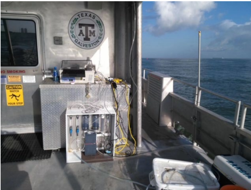
Figure 3 an underway CO 2 partial pressure ( p\text{CO}_2 ) system deployed on a sampling cruise in Galveston Bay during the NSF RAPID project
