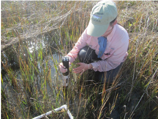
Using a bbe BenthosTorch to record benthic microalgal biomass
