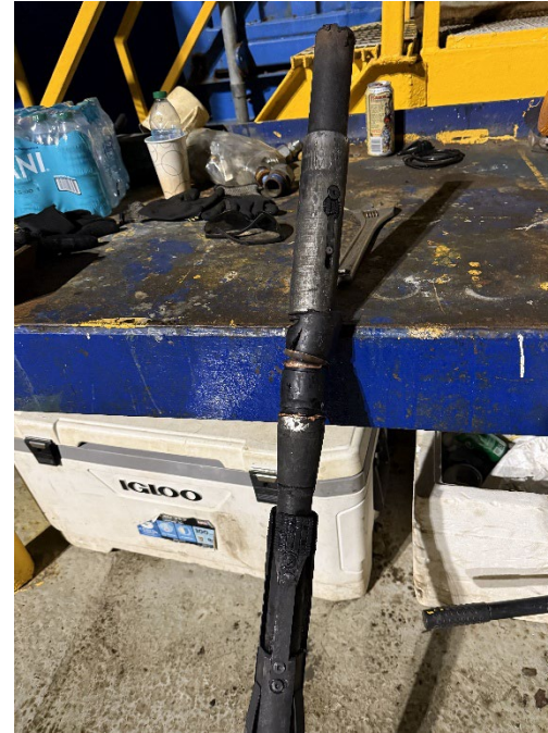
Leaking Packer Pulled
