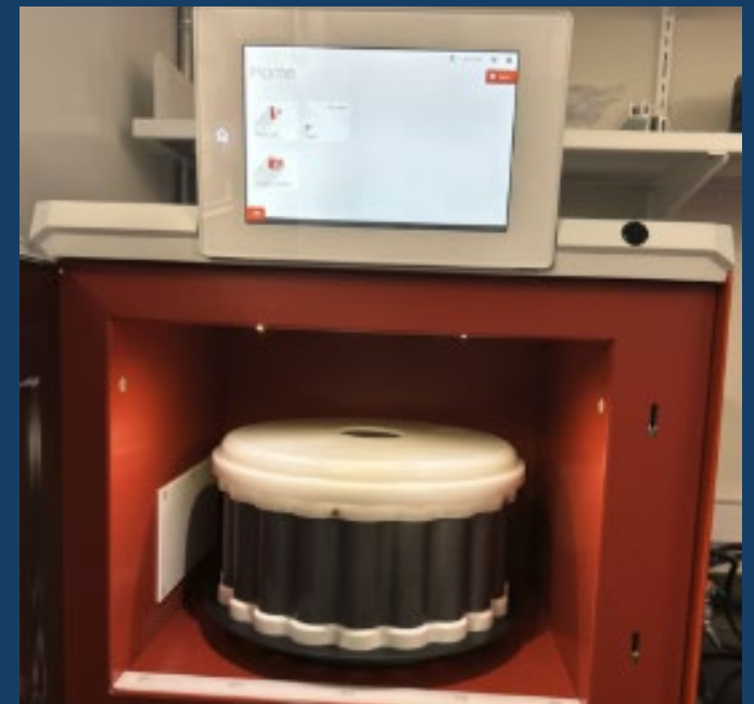
Closed Vessel Acid Digestion & Dilution
