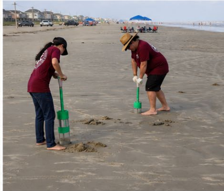
5. Collecting sediment cores for benthic community and contaminant analyses.
