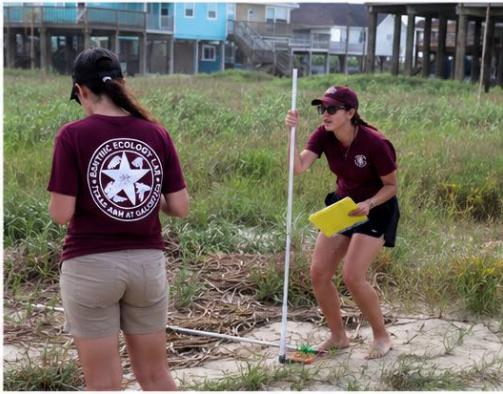
1. Measuring beach elevation and vegetation at a sampling site.
